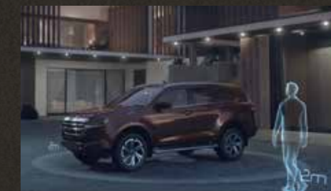
Welcome Light lights up the cabin when approaching the vehicle within a distance of 2 meters.
