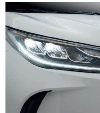
LED HEADLAMPS* The new headlamps of the Yaris were redesigned to accentuate the Daytime Running Lights, and lead your way in style.
